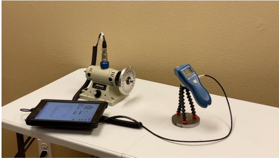
Figure 7 Single-Plane Two-Channel Balancing Setup
