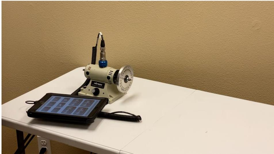
*Figure 4 Single-Channel Four-Run Balancing Setup*
