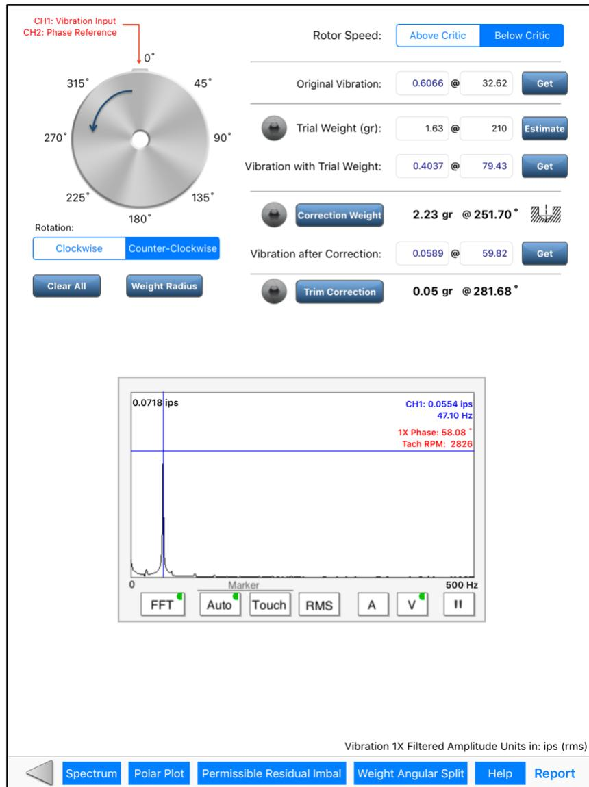
Figure 9 Single-Plane Two-Channel Balancing in iRotorBalancer App
