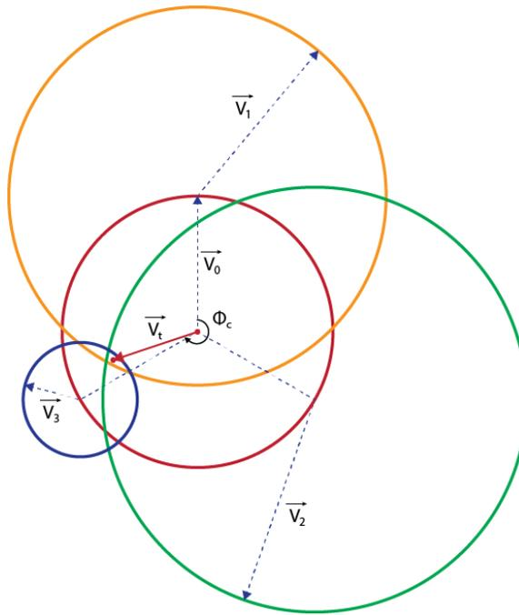
Figure 5 Single-Plane Four-Run Balancing Diagram
