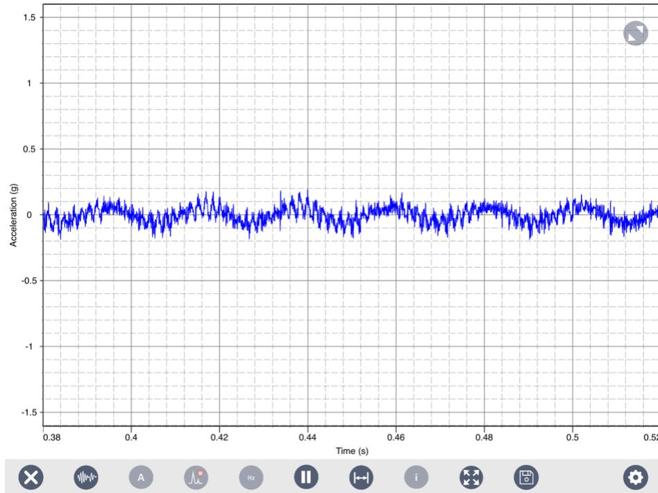
*Figure 12 Waveform After Balancing with Single-Plane Two-Channel Method*
