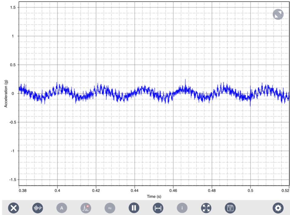
Figure 10 Waveform After Balancing with Single-Plane Four-Run Method
