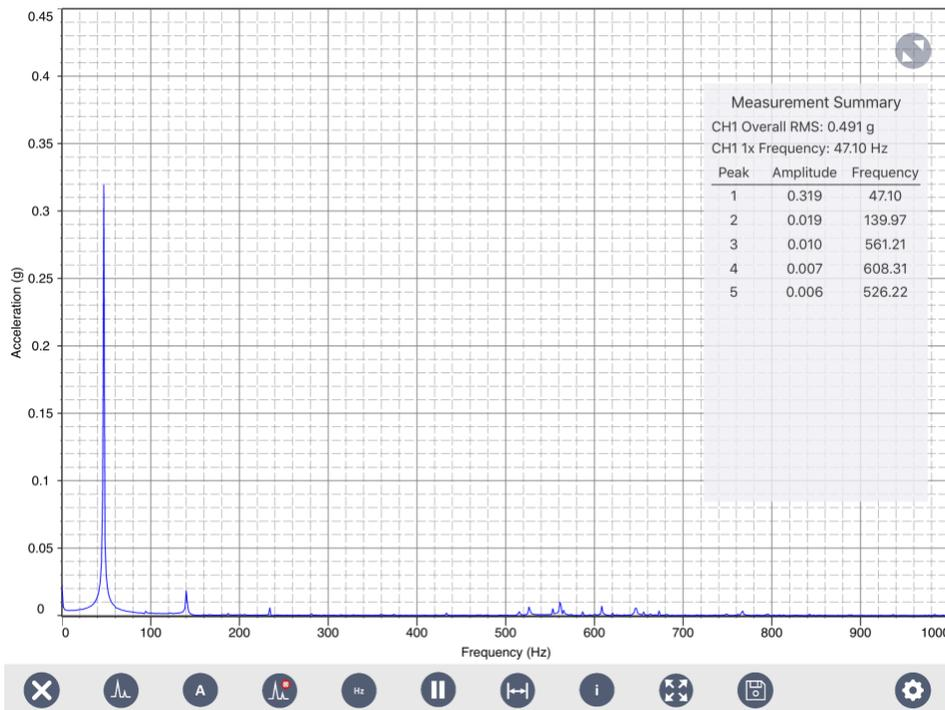
Figure 3 Spectrum Before Balancing
