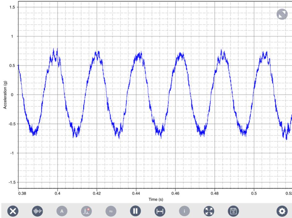
Figure 2 Waveform Before Balancing
