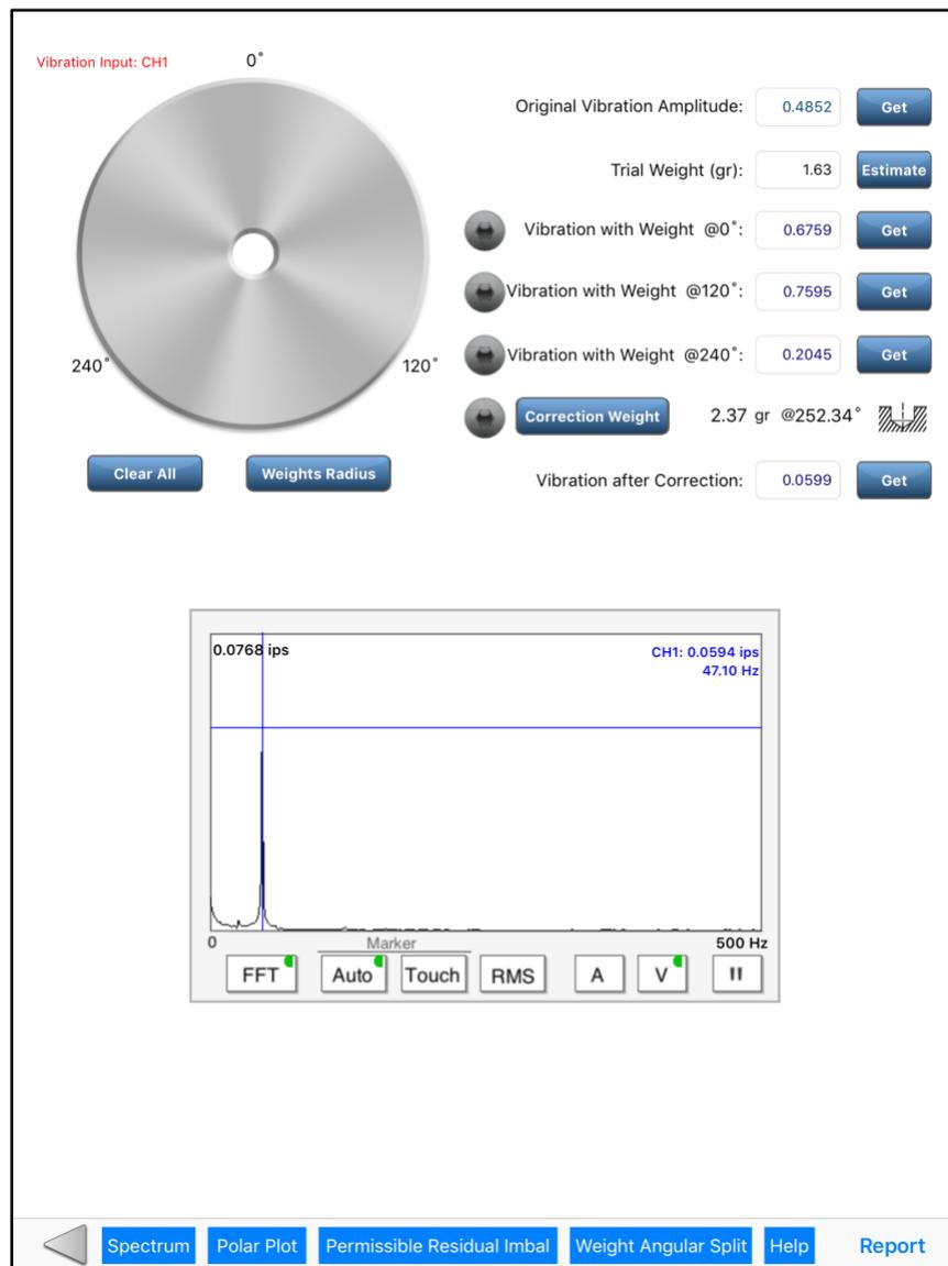
Figure 6 Single-Plane Four-Run Balancing using iRotorBalancer App
