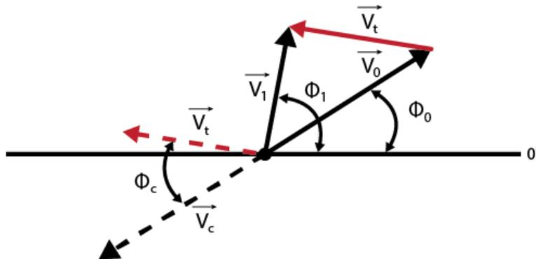
Figure 8 Single-Plane Two-Channel Balancing Diagram
