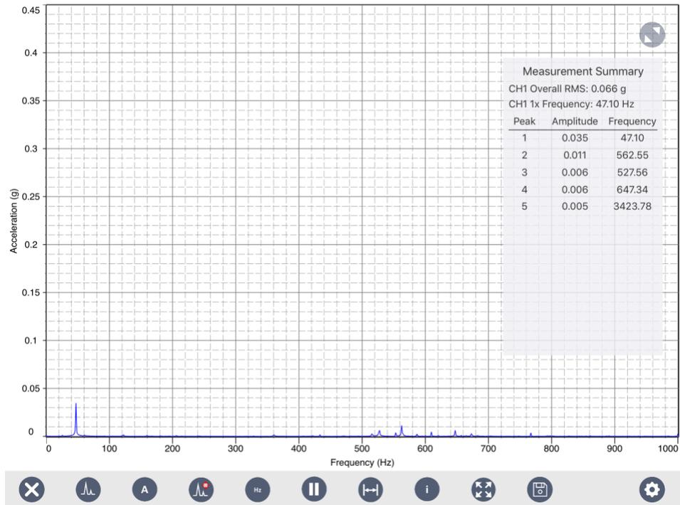
Figure 11 Spectrum After Balancing with Single-Plane Four-Run Method
