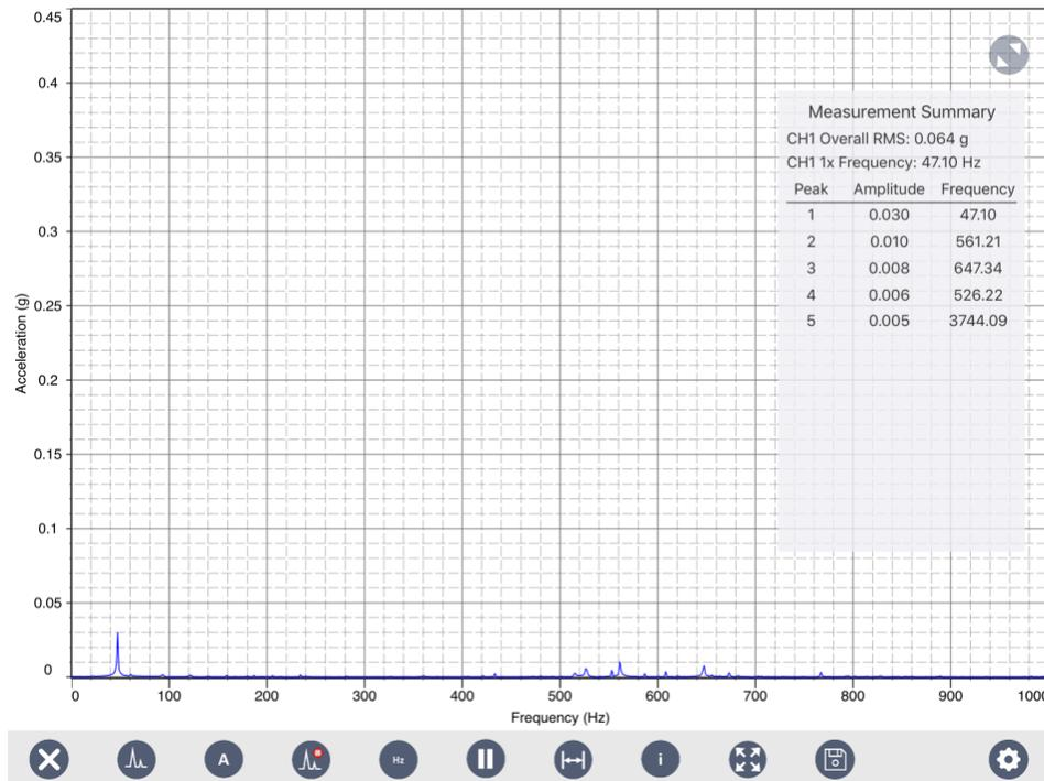
Figure 13 Spectrum After Balancing with Single-Plane Two-Channel Method
