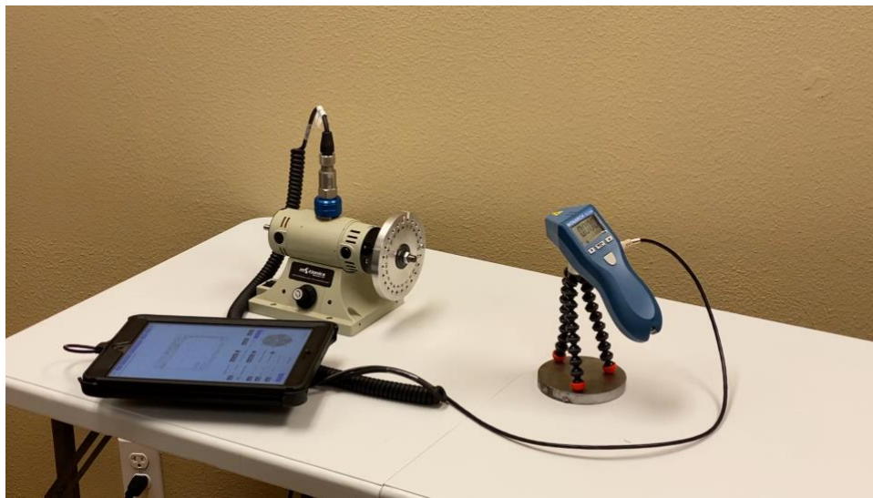
Figure 1 Single-Plane Two-Channel Balancing Setup
