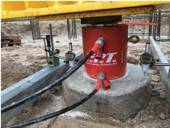
Fig. 1 Compression Load Test
