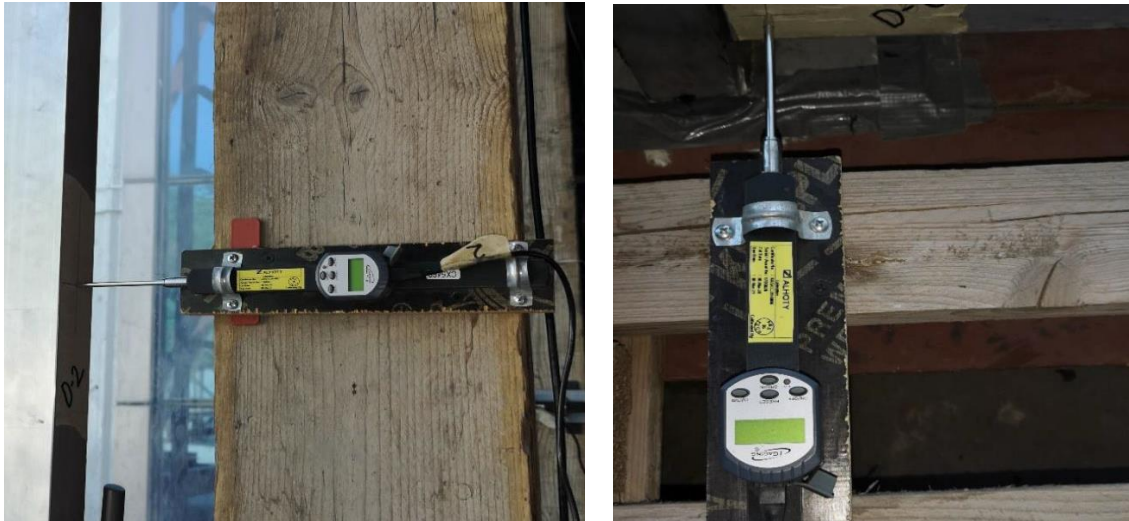
Fig. 4, 5 Motionics gauges used in multiple positions to record load deflections of aluminum mullions and transoms of a curtain walling system under pressure within a purpose-built test chamber.
