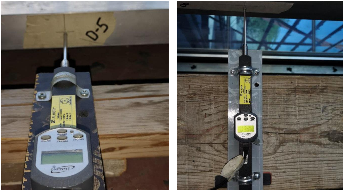
Fig. 2, 3 Motionics gauges used in multiple positions to record load deflections of aluminum mullions and transoms of a curtain walling system under pressure within a purpose-built test chamber.
