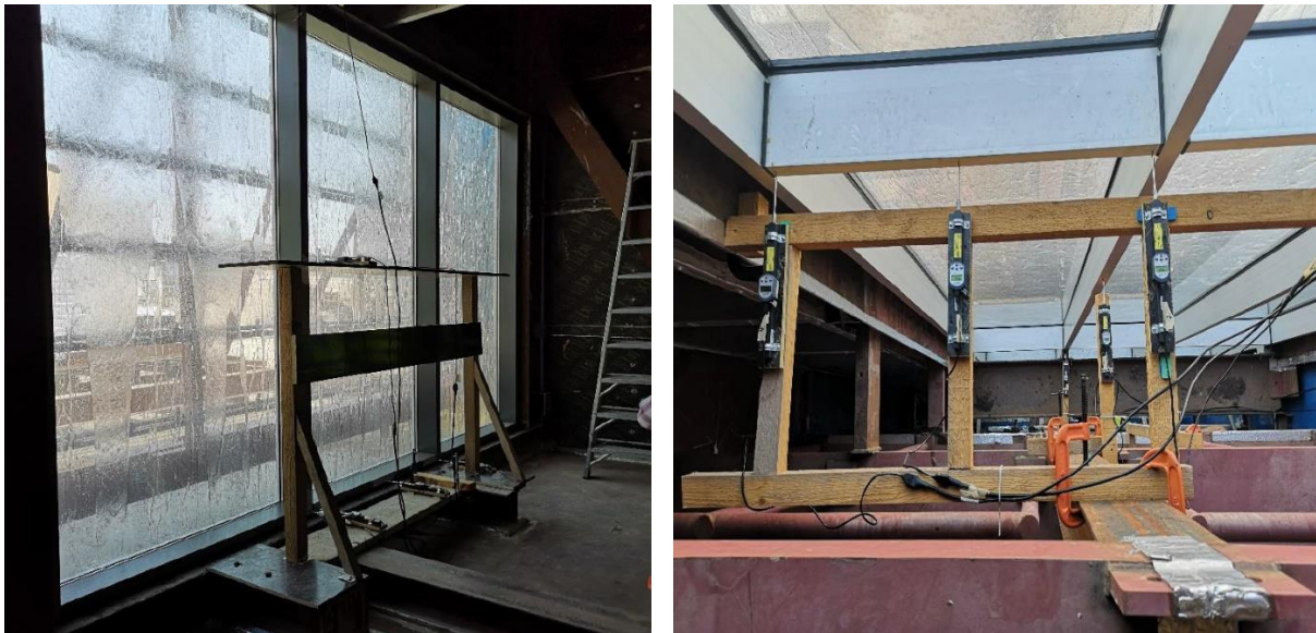
Fig. 6, 7 Motionics gauges were placed at heights of up to 12m in the testing chamber.
