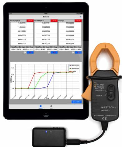
iWMD is a series of wireless measurement devices with high resolution. It allows the user to measure various sensor readings and communicate wirelessly with smart devices such as the iPad via Bluetooth Low Energy.
