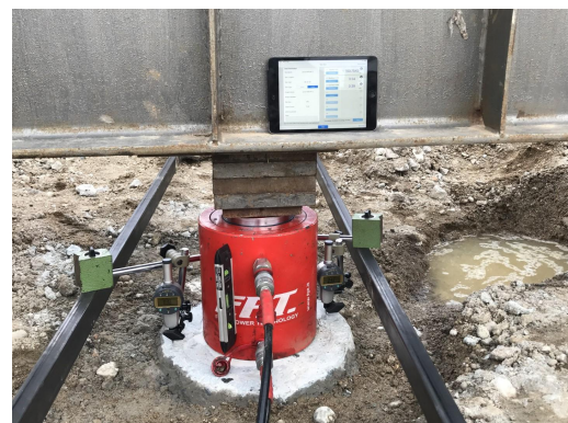
Fig. 6 App in use during pile compression test
