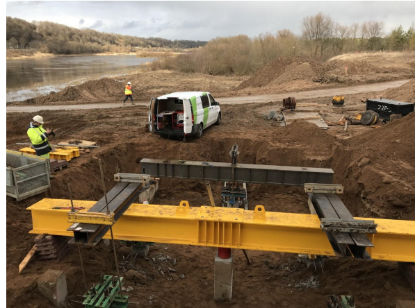
Fig. 3&4 Work site where pile load tests are conducted
