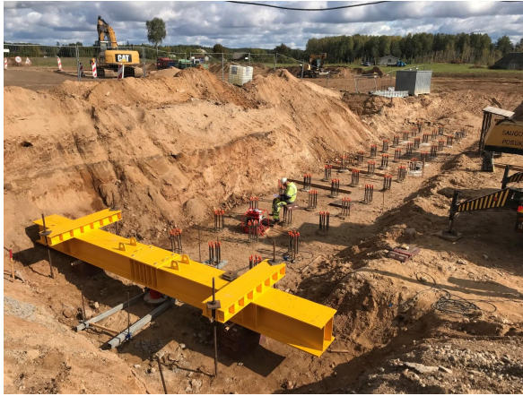
Fig. 3&4 Work site where pile load tests are conducted
