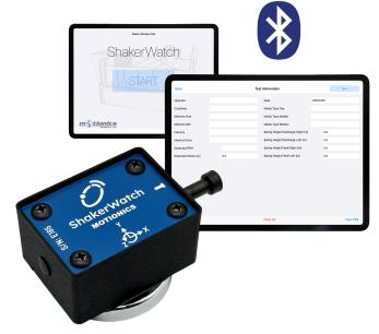
The ShakerWatch iPad app performs X-Y orbit tests with auto-calculated RPM, G-force, stroke and angle. Bump test, side displacement and support structure vibration tests can be also be performed within the app.
